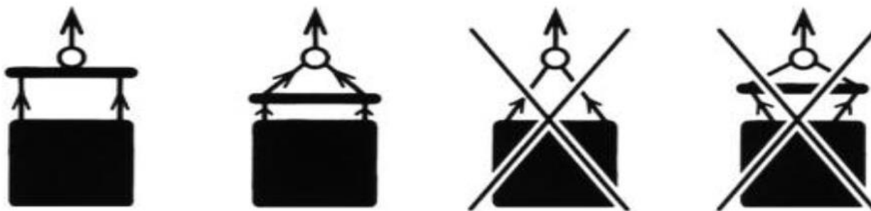
Figure #6 : La manutention correcte des micro stations BioKlar® ULTRA BKU10eh
