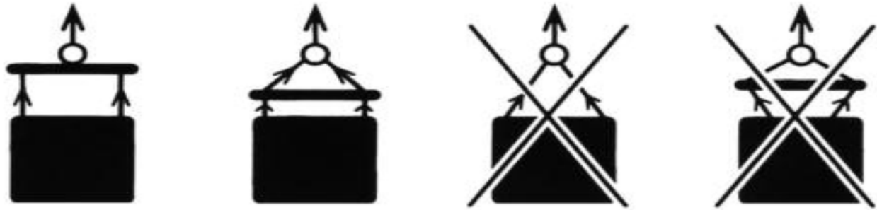
Figure #4 : La manutention correcte des micro stations BioKlar ULTRA
